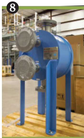
8 Planning single-phase and boiling tests with the new Tranter shell-and-plate welded heat exchanger
